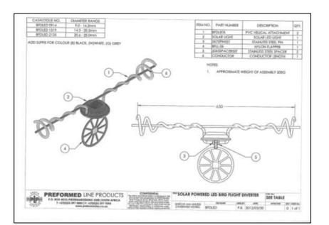
Figure 23: Solar-powered LED flight diverter<sup>28</sup>
